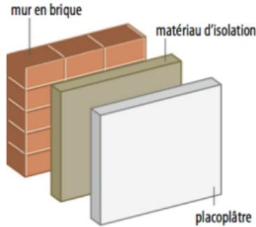
$$R_{th}^{\text{total}} = R_{th}^{\text{mur}} + R_{th}^{\text{isolant}} + R_{th}^{\text{placo}}$$
